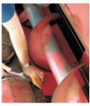
3. Insert the poly center panel under the auger as illustrated. IT IS VERY IMPORTANT TO PUSH THE POLY PANEL REARWARD UNTIL THE REAR EDGE OF THE POLY MAKES CONTACT WITH THE STRIPPER ANGLE AND THE FRONT EDGE "SNAPS" BEHIND AND BELOW THE FRONT STEEL RAIL OF THE HEADER. It may be necessary to use a block of wood to drive the panel into position as illustrated. NOTE: If necessary, raise the auger to maximum height. Readjust auger to desired height after installation is complete.
