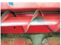
11. Locate the hole approximately ¾" from the front edge. Secure with ¼" -20 x ¾" truss head bolt. IMPORTANT: TIGHTEN THE NUT TO SEAT THE HEAD OF THE BOLT THEN LOOSEN THE NUT 3/4 TURN. THIS WILL ALLOW THE LINER TO EXPAND AND CONTRACT WITH TEMPERATURE CHANGE.
