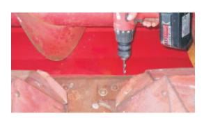
10. To complete the installation, drill a 3/8" hole at each row. Drill  $3\frac{1}{2}$ " – 4" left of the center of the row unit for all rows that are left of the center line of the header and  $3\frac{1}{2}$ " – 4" right of the center of the row unit for all rows that are right of the center line of the header. Confirm that this offset is correct to miss the gear box and clutch assembly on the underside. Drill from the topside downward.
